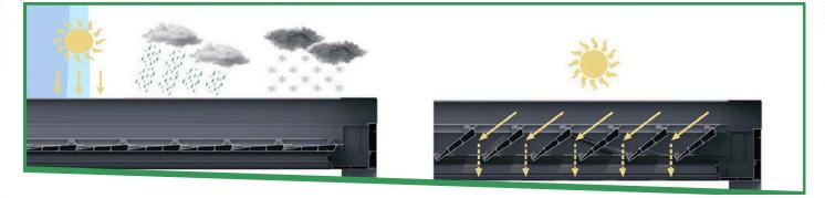
Provides protection from all weather conditions the roof remains closed
